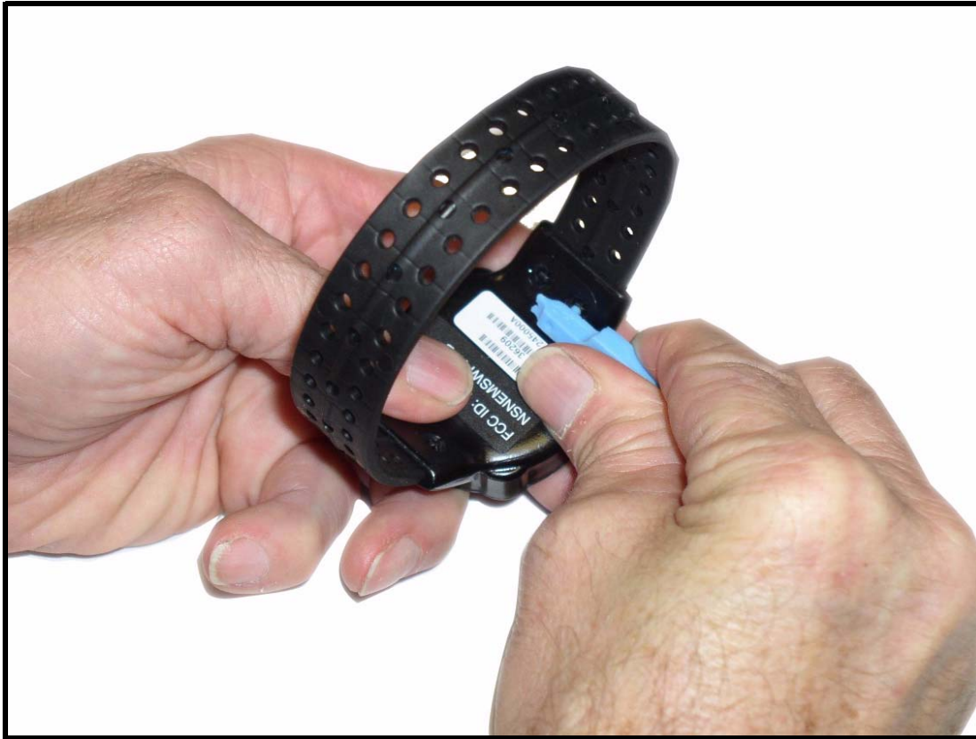
Figure 15: Using tool to elevate pin from underneath transmitter
