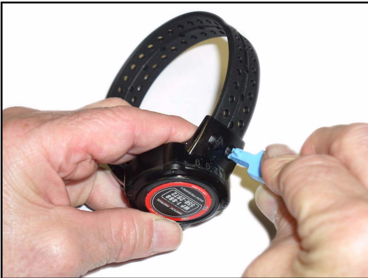
Figure 14: Inserting plastic tool to turn pin
